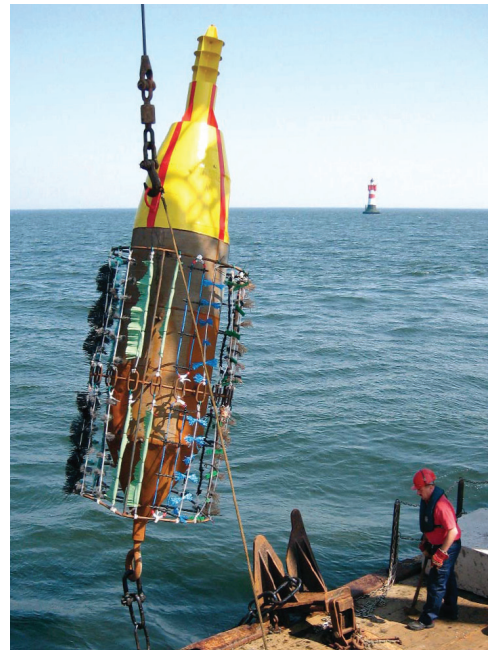
Fig. 4 Test buoy with different collector types deployed near the lighthouse Roter Sand [6]
