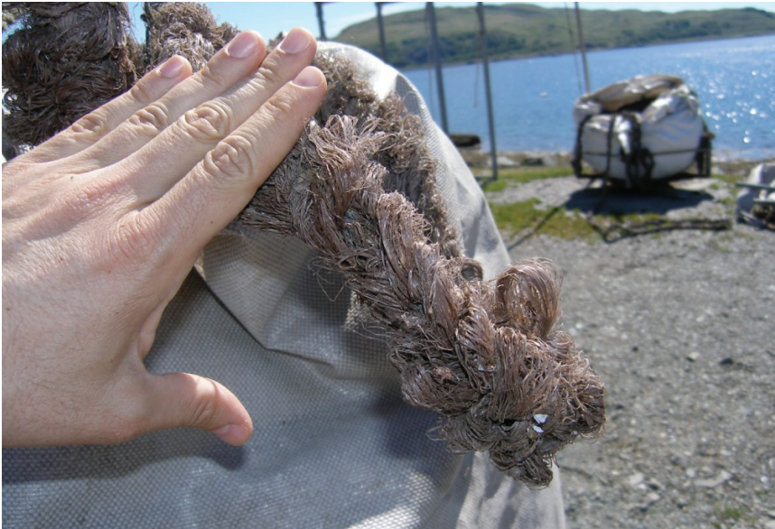
Figure 2. New Zealand rope, the rope is specially made to increase the surface of attachment for spats or larvae.
