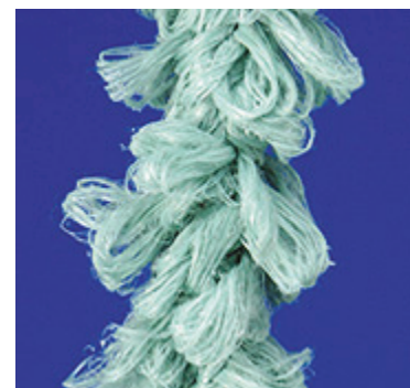
Figure 7; Open water crop rope
