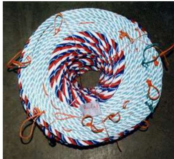
Figure 40: Coiled mainline rope ready for storage
