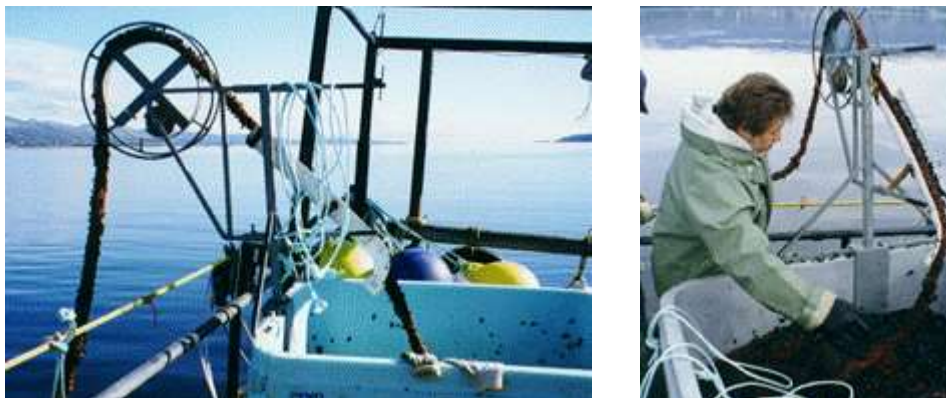
Figure 56 Hand-made mechanical wheel with a counter to measure collector rope length
