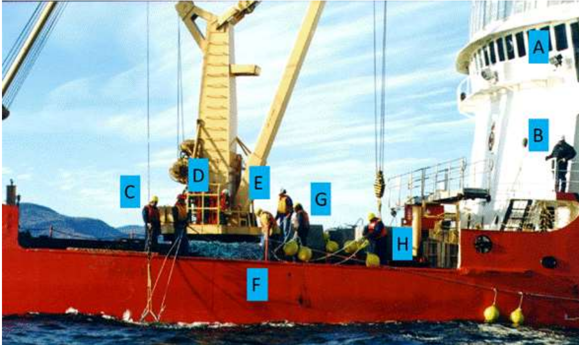
Figure 48 Deployment of the concrete anchors in a longline series from a big ship able to move 3 tons anchor
