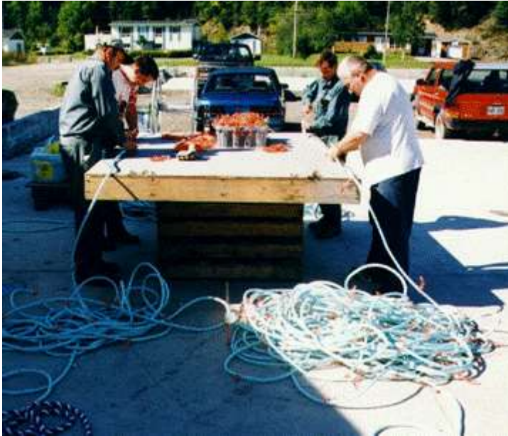
Figure 38 The Loop cord is easily inserted into the mainline with a splicing tool on the table when the rope is not under tension
