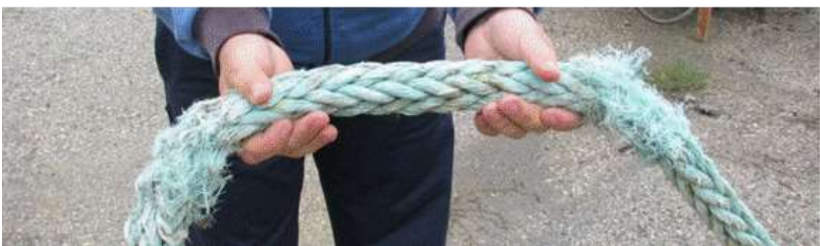
Figure 18 Consequence of using unknown rope material and mixing two rope qualities together
