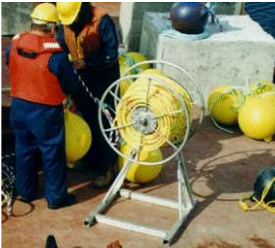
Figure 39: The mechanical rope coiler is used to coil the rope for transport and for deploying at sea
