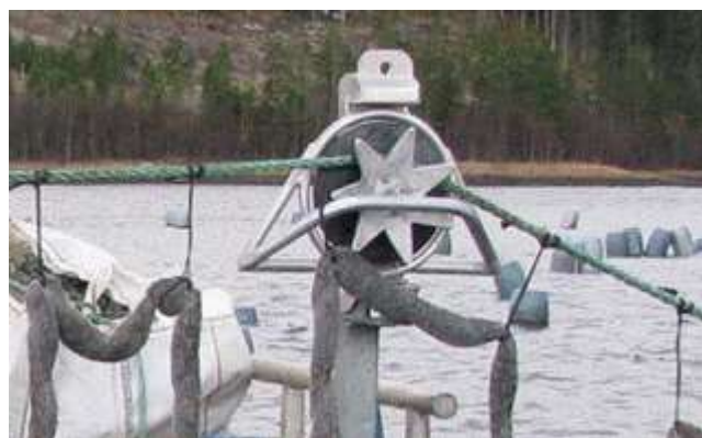
Figure 24 Mainline rolling through the starwheel
