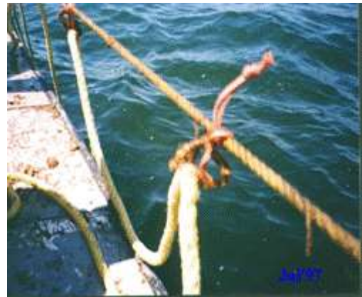
Figure 42 Continuous collector with short dropper is threaded through the loop cord and attached directly to the mainline
