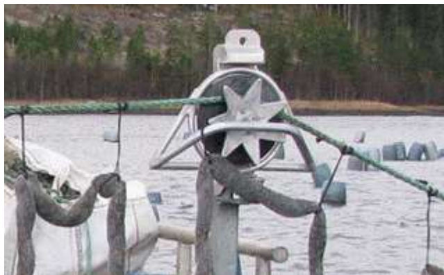
Figure 24 Mainline rolling through the starwheel
