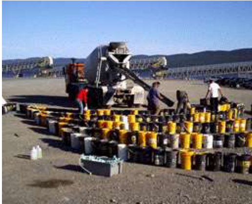
Figure 17 Production of compensation ballast weights
