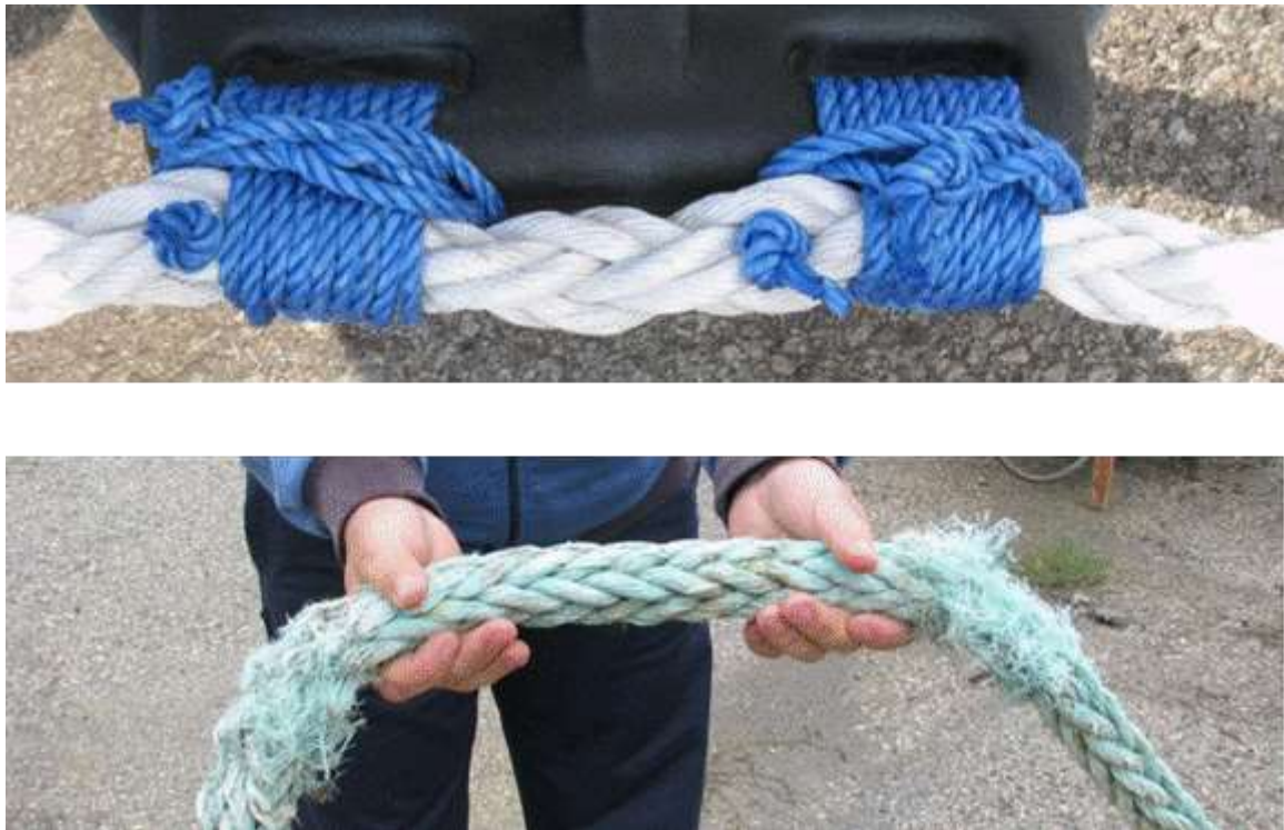
Figure 18 Consequence of using unknown rope material and mixing two rope qualities together
