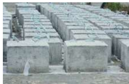
Figure 7 Unmoulded concrete blocks after using grease on inside of wooden moulds
