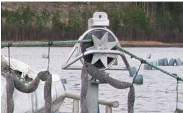
Figure 59: Starwheel set up on a mussel workboat
