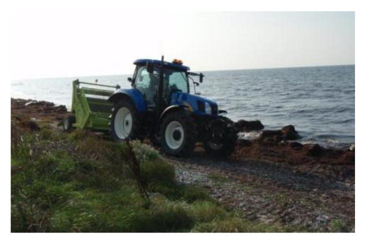
BeachBeachTech 2800 represents itself an example of such a cleaning machine. Its technical description reveals that volume of its garbage collection container comprises 2.8 m<sup>3</sup>. Such a volume is insufficient for serious algae harvesting projects since small size container must be unstuffed too often.
