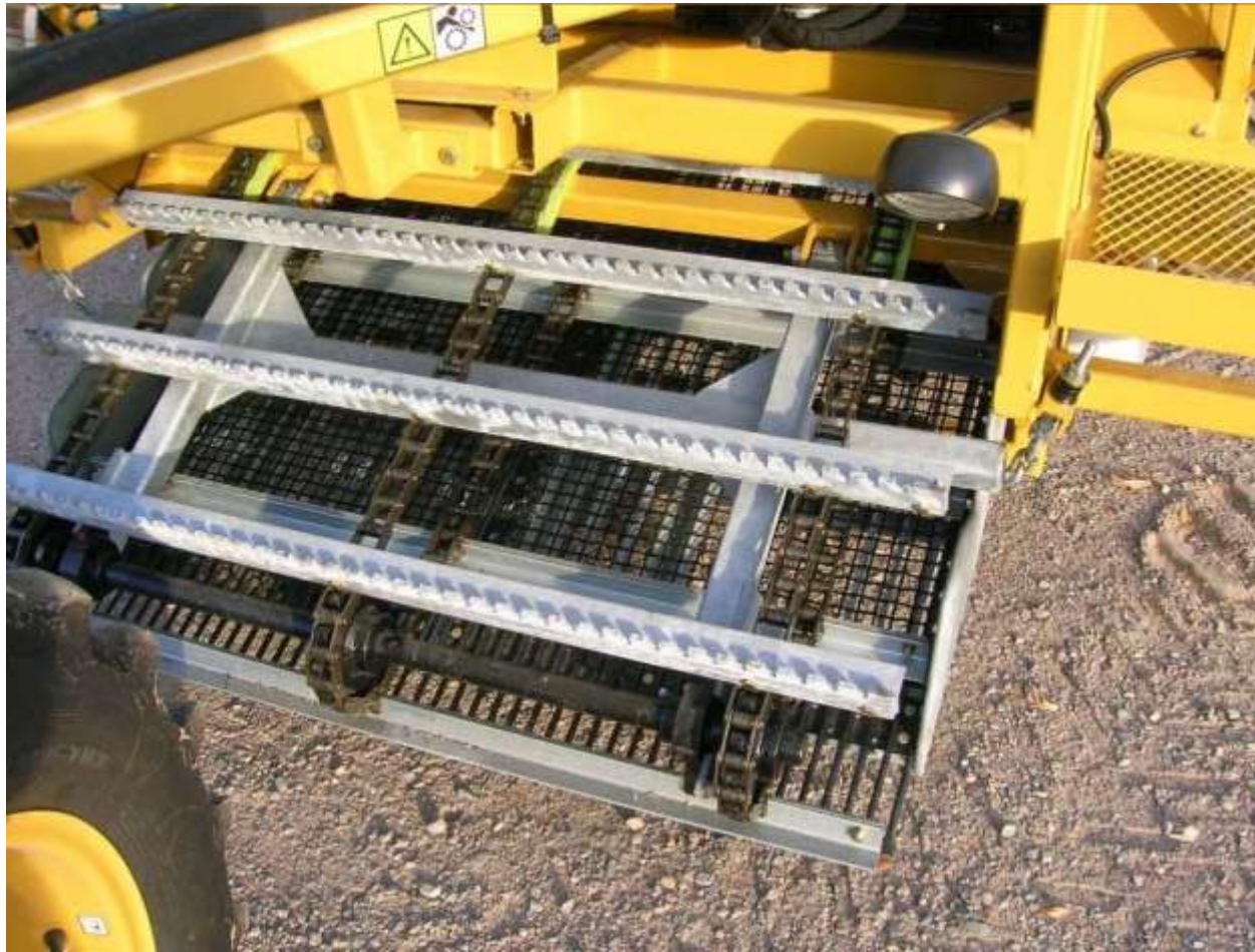
Fig. 9. “Cherrington” company’s garbage collection machine’s set-up 13
