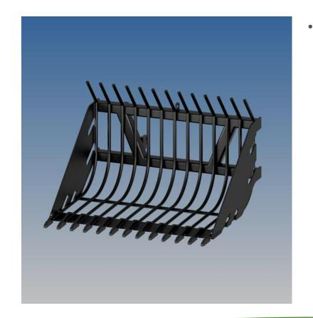
Improved bucked has 13 longer vertical branches. This improvement allows to enlarge the capacity of the bucket and increase overall efficiency of collecting Mounting fixtures comply to process. "Euro" (ISO 23727:2009) standard and allows fast mounting/unmounting of grate bucket. All metal parts are manufactured using CNC equipment, from hard steel alloy.
